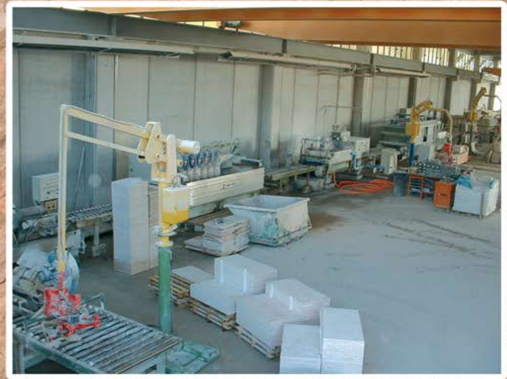
PRODUCTION LINE FOR EXTERNAL AND INTERNAL FLOORINGS We can see the machineries for the processing and the squaring of the tiles In the middle we can see the finished products
