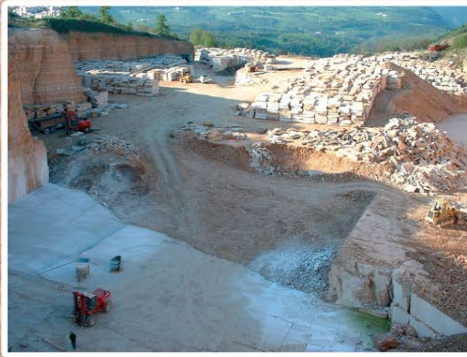
PARTIAL SIGHT OF THE QUARRY "SAN GIOVANNI LOFFA". WE CAN SEE THE SURFACE OF THE QUARRY WHICH IS BEING EXCAVATED AS WELL AS THE SLABS WHICH HAVE BEEN STORED AND WILL BE TRANSPORTED TO THE FACTORY TO BE PROCESSED.
